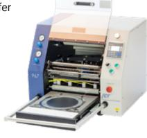
Crafted with the primary purpose of automatically affixing wafers onto tape, the ADT 967 Semi-Automatic Wafer Mounting System showcases a harmonious blend of intelligence and user-friendliness. This remarkable product holds significant value and is the ultimate selection for mounting during production processes.
