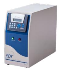
High quality processing, contamination-free devices ADT 947 CO2 Inline Injector is designed to eliminate particle adhesion and device damage caused by electrostatic effects. The units dissolve CO2 gas into de-ionized water (DI) used for dicing or cleaning processes, thus performing consistent control over an optimal level of resistivity.
